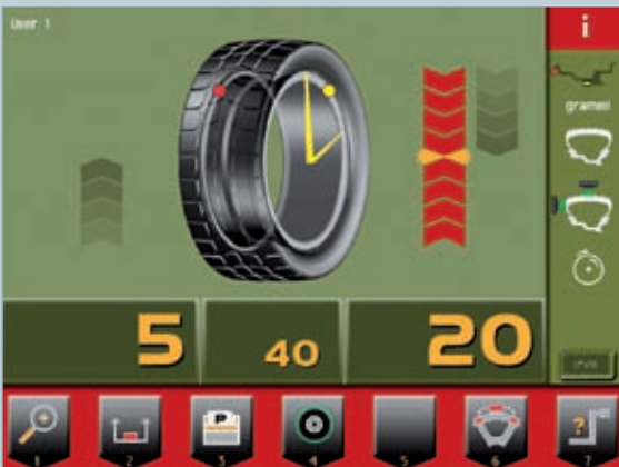
SPLIT program to divide counterweights between spokes of alloy rims.
