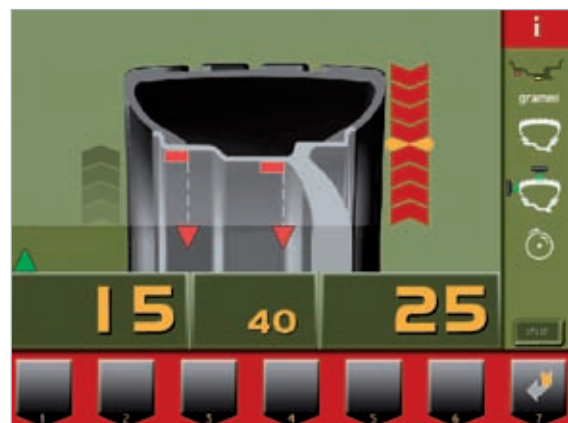
Axial position of counterweight displayed and indication of hidden positions for placing both adhesive weights.
