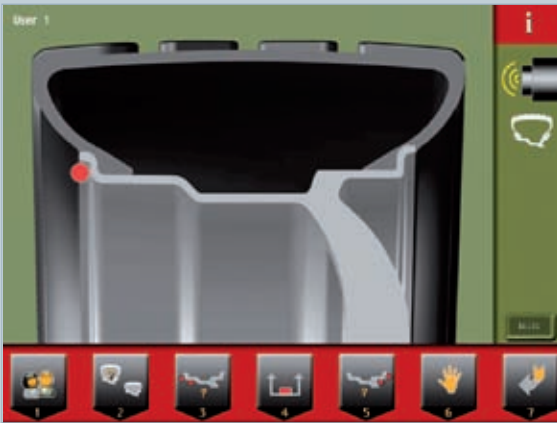
Automatic width measures with sonar (CEMB patent).
