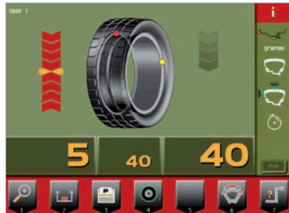
ALU-S function with "intelligent" gauge (automatic input of 2 diameters of rim/machine 2 distances) for correction of the wheel from inside.
