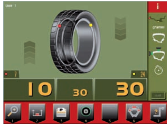
RPR function (Rear Planes Residual). It allows the simultaneous visualization of unbalance values: at the set correction planes, at the real correction planes (clip-on weight on rim edges) and in static mode.
