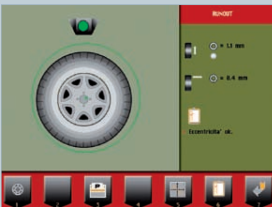
Eccentricity measuring system (1st Harmonic and Peak to Peak) with Sonar (option). It is automatically activated during balancing cycle allowing operators to get the information about wheel eccentricity without any time loss. Alarm alert if eccentricity is out of tolerance. Specifies procedure recommend to reduce the eccentricity.
