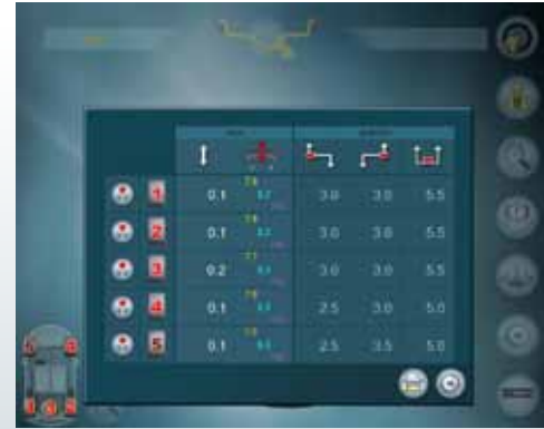
Measurement of wheel conicity with indication of side slip
