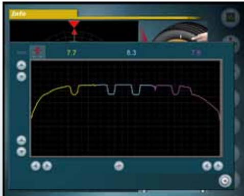
Measurement of wheel conicity with indication of side slip
