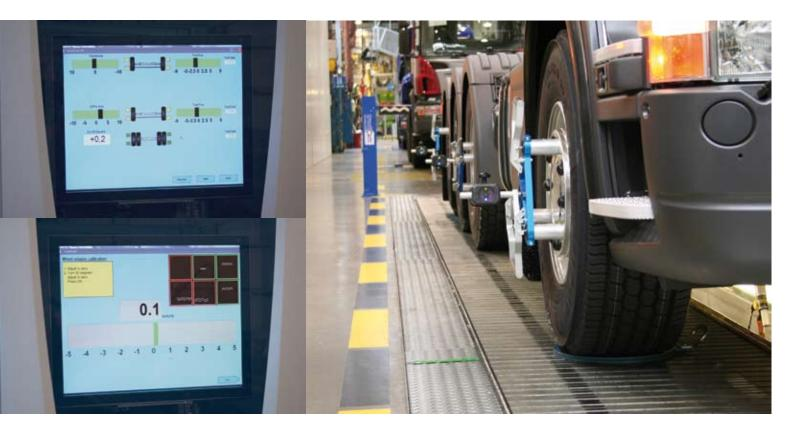
The system can be configured for all vehicle types with their different axle configurations, and target values as well as tolerances can be entered into the software. The adjustments can only be finished when all values are in tolerance. This ensures that every vehicle that leaves the production line is properly aligned.
