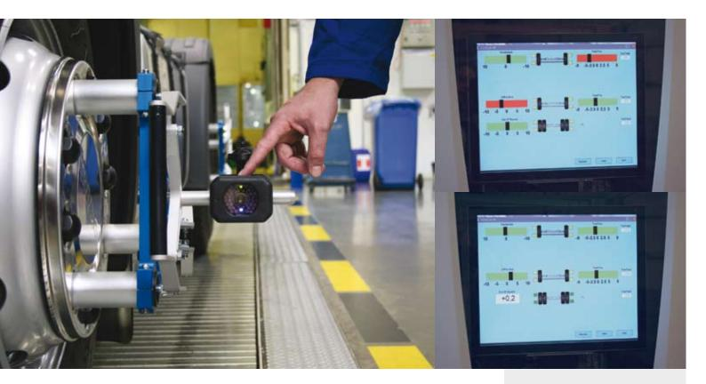
The actual measurement process starts as the operator aims the camera forward, clicks the OK-button, turns the camera over pointing backwards and clicks again. This click-turn-click procedure is done once for each wheel, giving the software enough input to calculate angles like toe, out of square and parallelism. Parallelism of all axles is calculated with the rear axle as reference.
