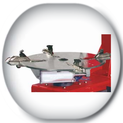
Self-centring turntable with two clamping cylinders (plastic protectors are optional extras).
