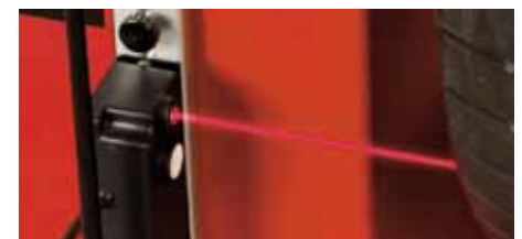
Sonar LR: no contact lateral eccentricity measure.
